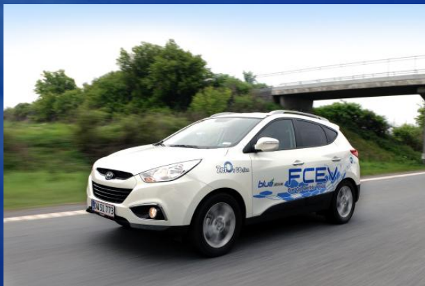
■ Crossing Denmark: 340km on single H 2 charge (May)
