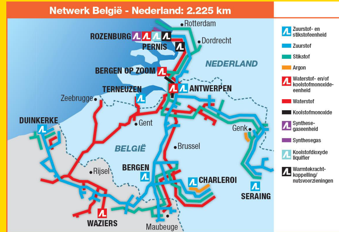
Pipeline network of Air Liquide, hydrogen in RED
