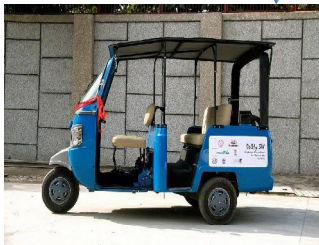
Figure 21. Hydrogen Fuelled Passenger 3 Wheeler
