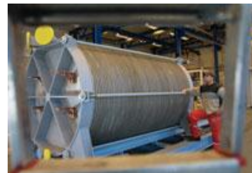
Norsk Hydro Large Electrolysis Stack (975 kg/day)
