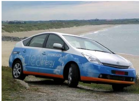
15 Toyota Prius Converted to ICE Hydrogen by Quantum (US) Range: 170 km
