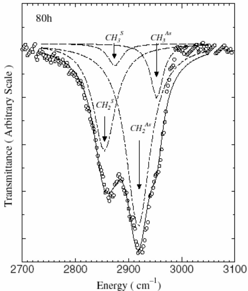
H atom can be absorbed as -CH<sub>3</sub> or -C<sub>2</sub>H<sub>5</sub> in C<sup>nano</sup>H<sub>x</sub>
